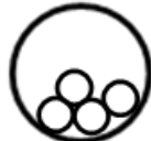
4 cables, Cradled; D/d \geq 3.0
