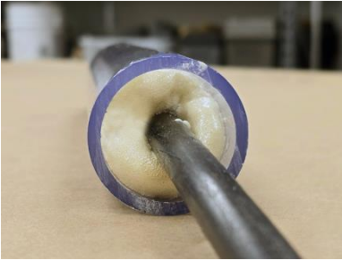
Replace static mixer with plug
