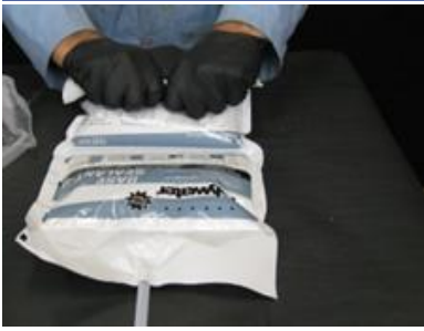
Burst primary seal
